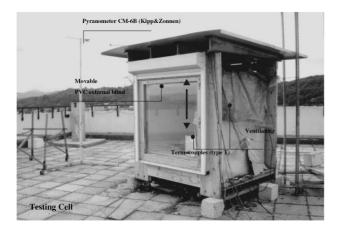
Fig. 10. Picture of testing cell.
